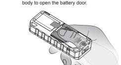
Insert 3, 1.2V AAA batteries according to the direction icons on the inside of the battery compartment. The TPE sealing ring has been
