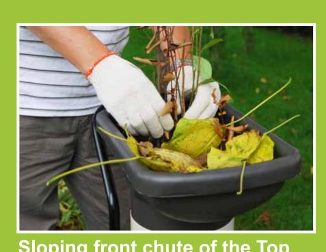
Sloping front chute of the Top Hopper is designed to accept leaves and small garden clippings
